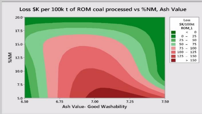
Contour plot showing the performance (loss \$k per 100k of ROM coal processed versus the percentage NM, ash value) of a “good” coal. The redder the colour, the higher the loss. Optimum operation will be found in the darker green colour regions of the plot.
