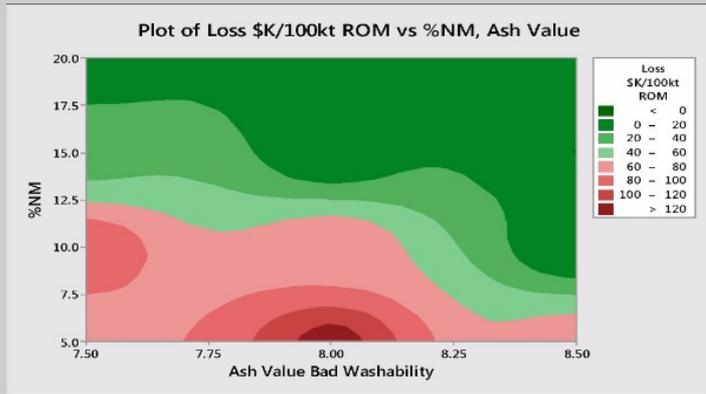
Contour plot showing the performance (loss \$k per 100k of ROM coal processed versus the percentage NM, ash value) of a “bad” coal. The redder the colour, the higher the loss. Optimum operation will be found in the darkest green colour regions of the plot.
